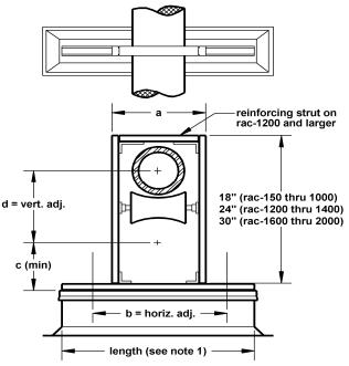
IMPORTANT: All fasteners must be torqued to 40 ft./lbs.
