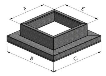
Difference between Existing Curb OD and New Fan Flange ID: greater than 1" and less than 6".
