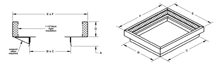
Options: galvanized, aluminum, stainless steel, damper ledge, access door, liners, vents
